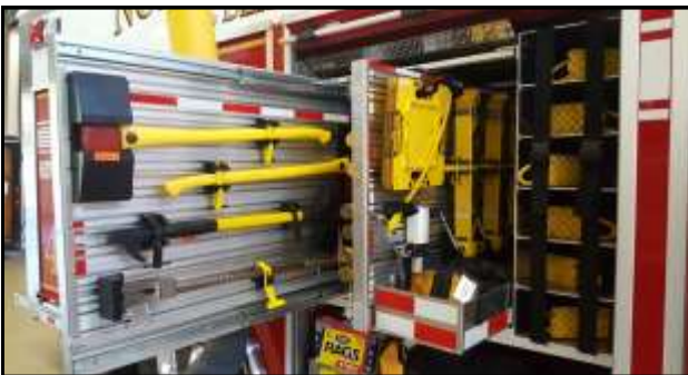
The forcible entry/ vehicle stabilization tool boards, located on Rescue 473.
