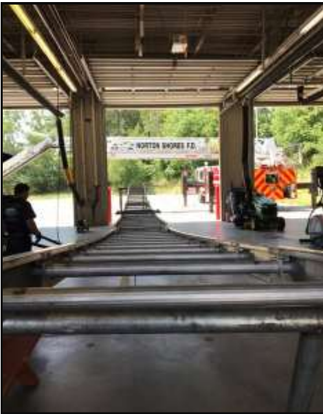
This extension ladder is being stress tested in accordance with NFPA standards.
